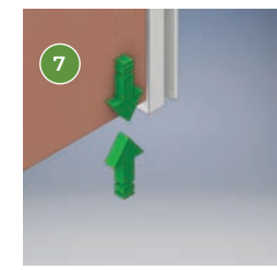
7 Threshold gaps are machined to suit your floor finishes and build program whilst ensuring that the essential 7mm required for fire doors is not exceeded. (3mm on smoke doors without dropdown seals).
