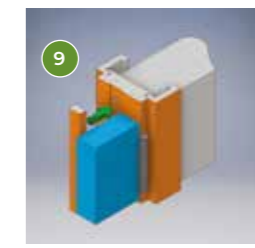
9 Frame fixings locations are pre-drilled in the correct location for fire certification and are hidden by the door stop.
