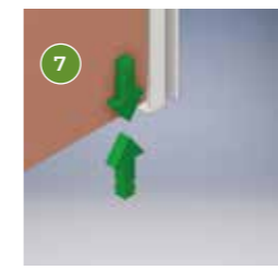
7 Threshold gaps are machined to suit your floor finishes and build program whilst ensuring that the essential 7mm required for fire doors is not exceeded. (3mm on smoke doors without dropdown seals).
