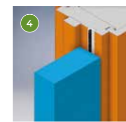
4 A 3 degree leading edge is machined on the lock side of each door to assist closing against smoke seals. (Single leaf doors only).
