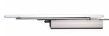
Size 2-4 Concealed Closer with Integrated Back Check Closing force variable by means of an adjustment screw. Adjustable closing speed and latch action. CE Marked and Certified approved. Cushioned limit stay available.
