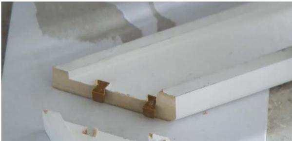
The Hoffmann fittings provided allow the joiner to effortlessly assemble the architrave sets, whilst providing a very tight mitred joint.
