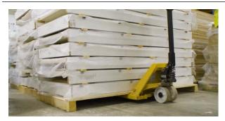
The Doorsets are delivered to site palletised to suit your build program (typically 6 to 7 Doorsets per pallet).
